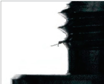
Mounting Post using TECHSPEC® 1X SilverTL™ Telecentric Lens and Standard Diffuse Backlight.
