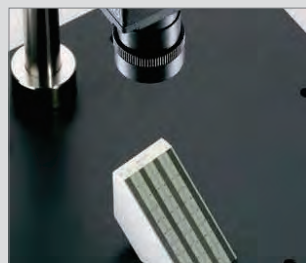
Figure 8: A depth of field target should be at 45° from the lens.
