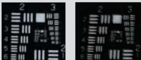
Figure 3b: The center and corner of an image that features balanced focus across the entire field.
