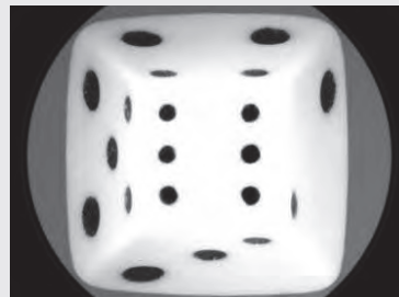
Images of dice using a Hypercentric Lens (left) and a Fixed Focal Length Lens (right).
