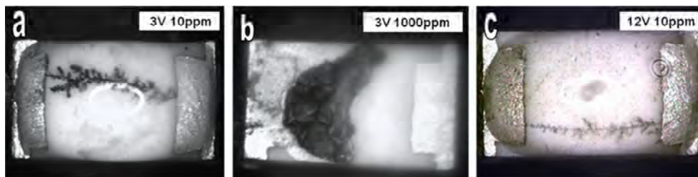
Figure 8.4: Effect of chloride and potential on the ECM of tin during experiments using chip resistor: (a) 3V, 10 ppm, (b) 3V, 1000 ppm, and (c) 12V, 10 ppm. (Anode is on the left and cathode is on the right). Dimensions of the components are 1.5x0.8mm (0605 housing).
