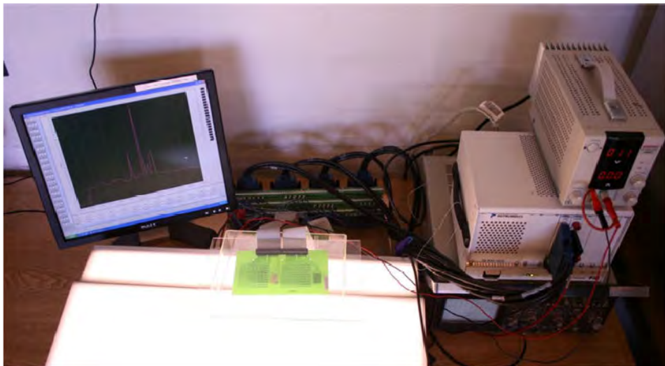
Figure 9.5: CELCORR test PCB setup for PCB level corrosion testing.
