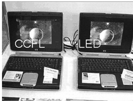
Figure 8.24 Display with conventional backlighting (left) and with LED backlighting (right).
