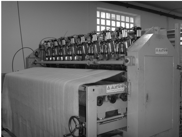
12.5 Wide format (up to 3 m) ultrasonic drum welding machine used for quilting.
