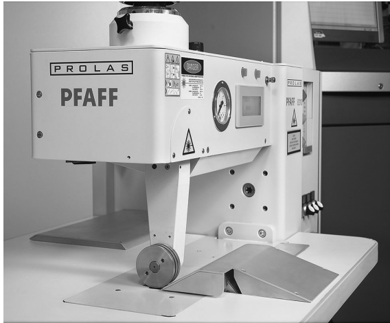
12.2 Continuous ultrasonic wheel welding and cutting machine (note this machine also includes laser welding).
