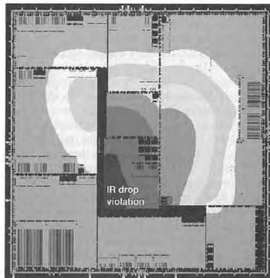
Figure 1.17 Contour plot of IR drop on a digital IC. Plots courtesy of Simplex Solutions, Inc.
