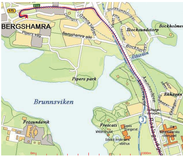
Fig. 6. Estimated trajectory (blue solid line) and GPS-receiver position estimates (red crosses) from the field-test. The vehicle was kept stationary (see top) for the first 30 seconds and then drove along the highway southward.
