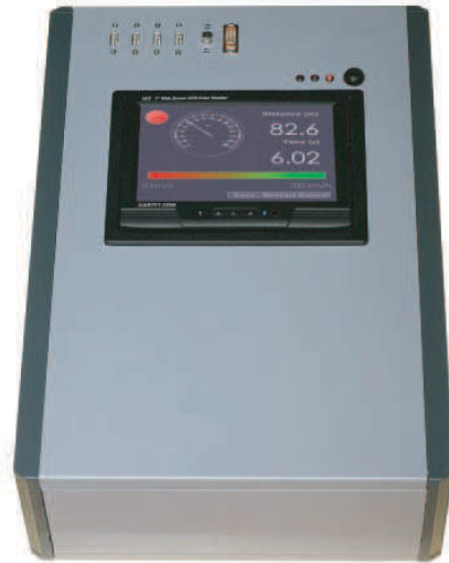
Fig. 1. The front of the navigation platform with its touch screen. In the upper left corner there are four USB-, a RCA- and a RS232 serial-connector, for connection of external sensors, an external screen and a GPS receiver, respectively.
