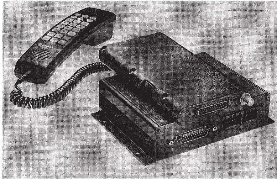
Figure 10.7 In-vehicle hardware components of the RESCU mayday system.
