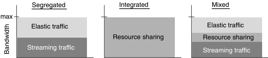
Figure 8.8 Ways of handling different traffic types
