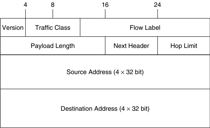
Figure 9.5 The contents of an IPv6 header
