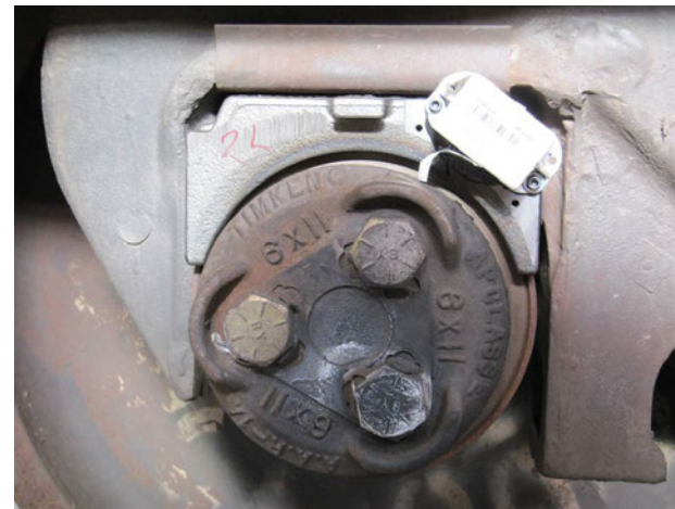
“2 bolt attached sensor (for larger bearing end caps)”
