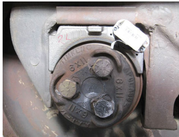
“2 bolt attached sensor (for larger bearing end caps)”
