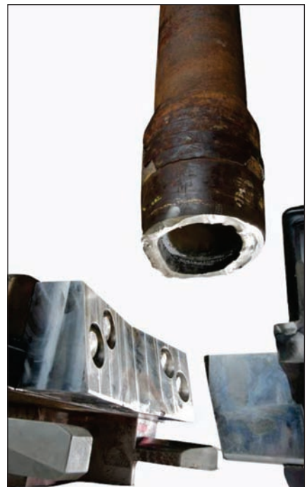
The blades of GE Oil & Gas' new blind-shear ram are designed to apply force and shear more effectively.
