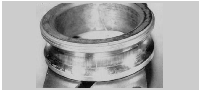
Fluting caused by internally generated current.
