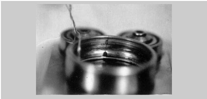
Fatigue Fracture of outer ring caused by burrs in the housing bore. Fig. 25
