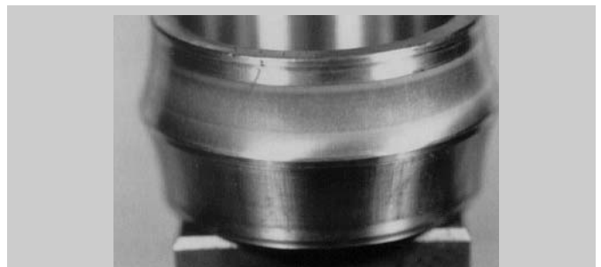
Excessive thrust on a Spherical Roller Bearing. Fig. 29
