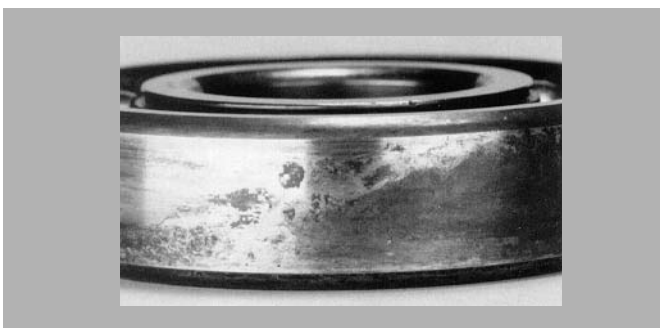
Fretting Corrosion caused by loss fit & vibration
