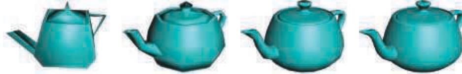
Figure 3.10. The effect of varying the tessellation factors. The Utah teapot is made of 32 patches. Inner and outer tessellation factors, from left to right, are 1, 2, 4, and 8. (Images generated by demo from Rideout and Van Gelder [1493].)
