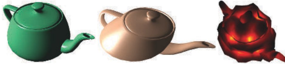
Figure 3.8. On the left, a normal teapot. A simple shear operation performed by a vertex shader program produces the middle image. On the right, a noise function creates a field that distorts the model. (Images produced by FX Composer 2 , courtesy of NVIDIA Corporation .)
