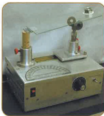
The Modified Chatillon Device measures the slip index.
