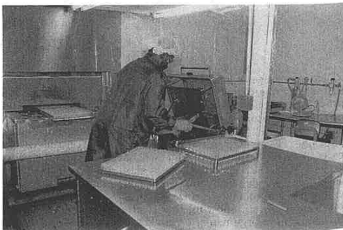
Fig 15. Cleaning vials with rack-loading washer, permitting handling vials by a full rack. After multiple-washing treatments, the racks are placed directly on the conveyor belt of the hot-air sterilizing tunnel (courtesy, Merck).
