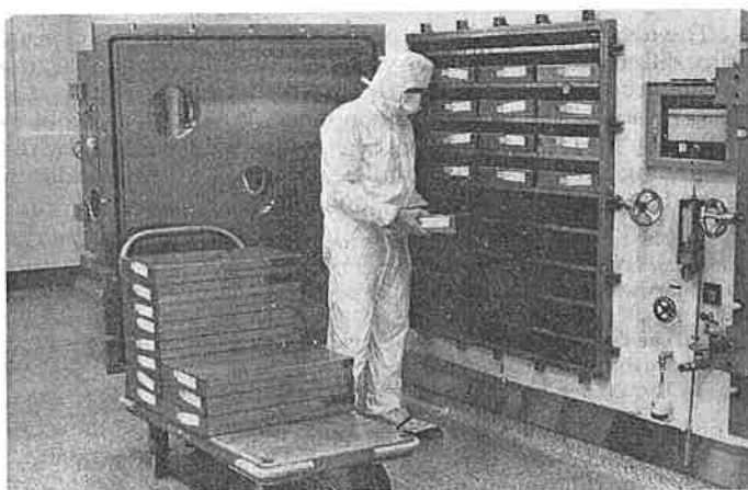
Fig 27. Aseptic loading of freeze-drier (courtesy, Upjohn).
