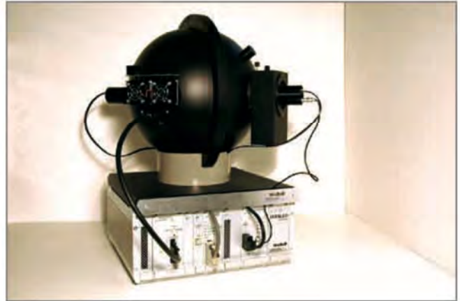
Figure 6: The TERALED extension for the T3Ster thermal transient tester provides high accuracy experimental radiometric and thermal data of LEDs
