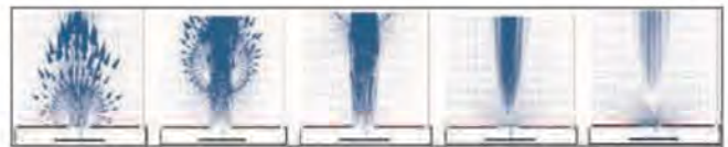
Figure 1: Particle image data showing the formation of a synthetic jet
