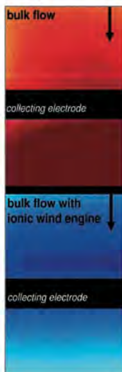
Infrared image of cooling with ionic "wind engines".
