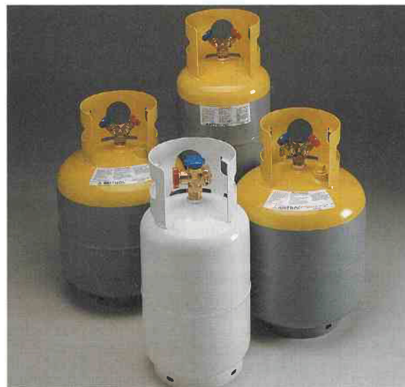
Figure 15-17. Recovery cylinders have gray bottoms with yellow shoulders and tops. Refillable-type cylinders, like the one in the foreground, may have solid colors. (Amtrol)
