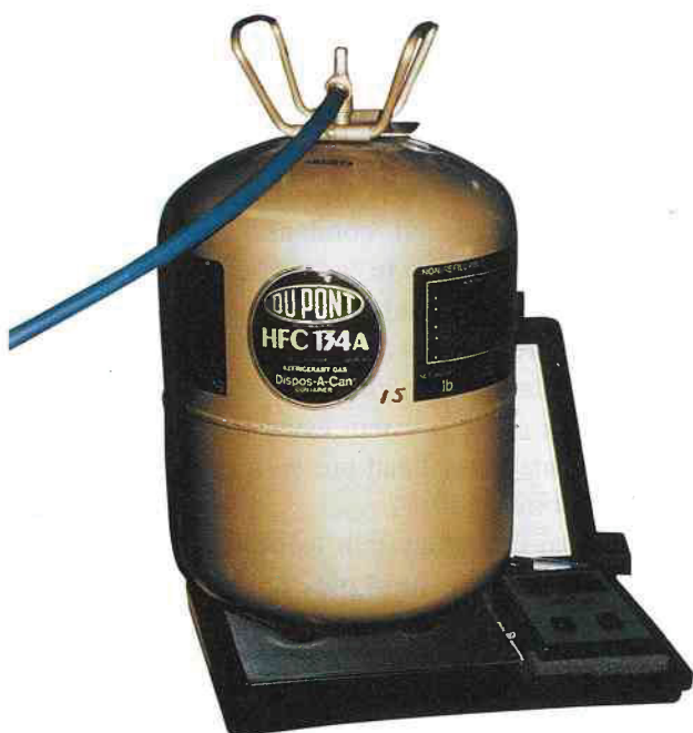
Figure 15-30. Electronic scales permit very accurate measurement of refrigerant while charging. The cylinder is placed on the scale pad, and the weight readout is adjusted to zero. As refrigerant is charged into the system, the readout will keep a running total in pounds and ounces. (TIF)
