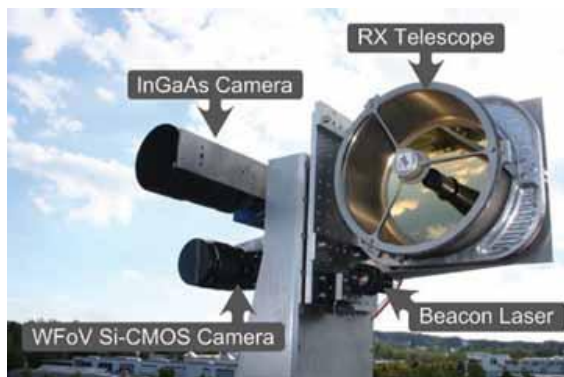
Figure 2. The optical ground station includes a 500mW beacon, InGaAs tracking camera and 200mm telescope positioned on an azimuth/elevation mount. The wide field of view (WFOV) camera is only used for demonstration purposes. RX: Receiver.
