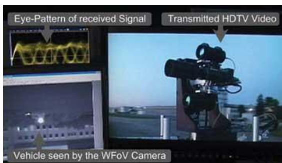
Figure 3. Successful mobile optical data transmission was achieved over 1900m at 1.5Gbps. The image shows the transmitted stream from the high definition television (HDTV) camcorder (right), the moving van with an 800nm test-beacon shown by the wide field of view camera (lower left) and the eye-pattern of the received signal (upper left).
