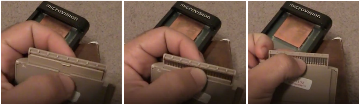
Closeup of Microvision cartridge attachment structure 6
