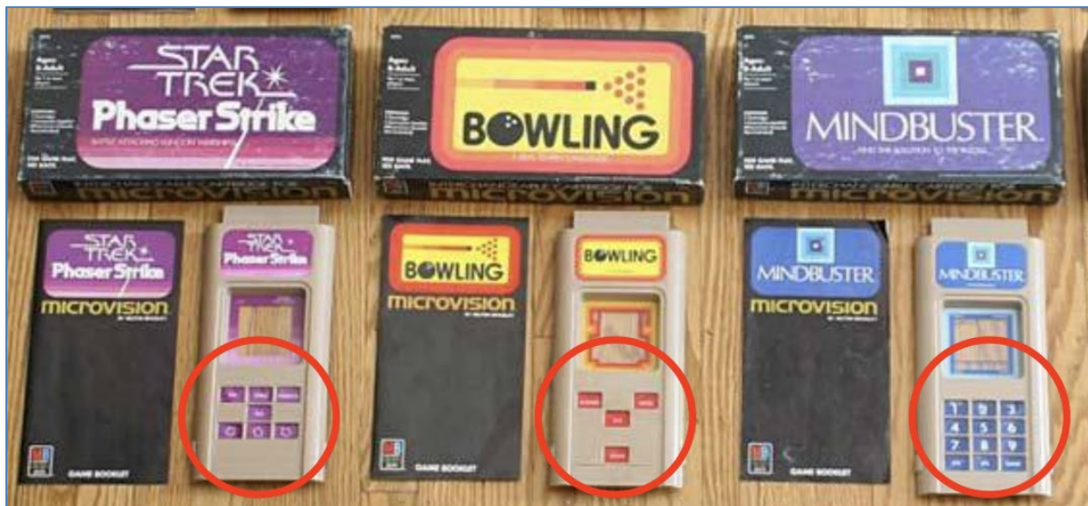
Microvision game cartridges with swappable input devices 5
