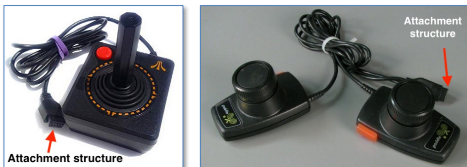
Atari 2600 game controllers using common attachment structure 3, 4
