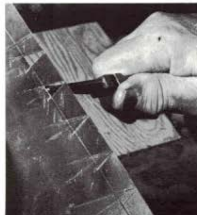
C. Breaking out the waste.
