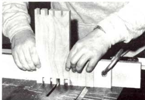
Once marked out, the pins are formed by wasting the wood between with dado-blade cuts. In the photo below, Duginske completes the second series of pin cuts.
