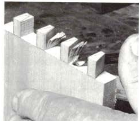
K. Cleaning pin bases with spear-pointed chisel.
