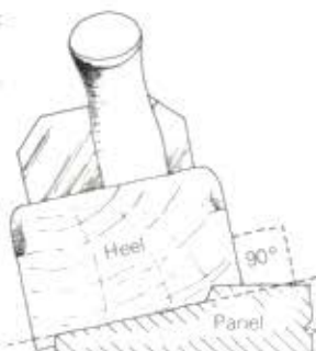
Sprung raising plane is held at 90° to bevel surface.
