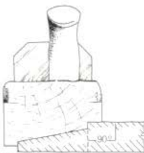
Shoulder angle of 90° is possible on planes used for a single panel thickness.
