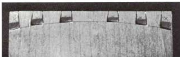
Fig. 3: Cutting the inside curves
