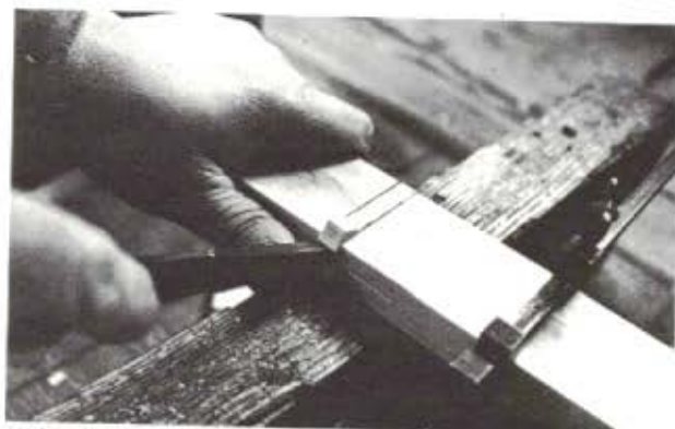
To break out the waste Odate pulls the corner of a flat chisel along the kerf (top). Then he clears the waste with a mortise chisel run in the notch, bevel-side down (above).
