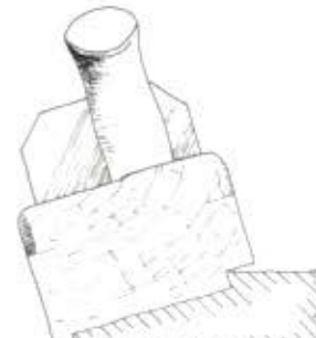
...but on thicker stock such a plane undercuts the shoulder.
