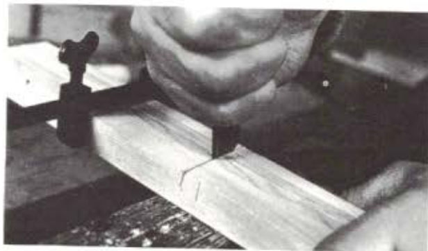
Odate clamps the kumiko (the thin strips that form the shoji grid) together in a stack and saws the notch shoulders a hair more than half-way through. A piece of scrap starts the saw correctly.
