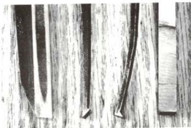
The tategu-shi 's mortising tools. From left to right, a mortising chisel, with hollow-ground face ( ura ); a mori-nomi , whose barpoon-like hook is tapped down and jerked up to remove chips; and a sokozarai-nomi , which scrapes the mortise bottom flat and also lifts out chips. Last is a steel rod for tapping flat the bottoms of small mortises.
