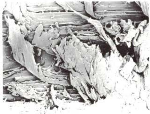
which allow liquid glues to penetrate. The partially detached fibers of a sawn surface, right, limit glue absorption to top layers and break readily under stress.
