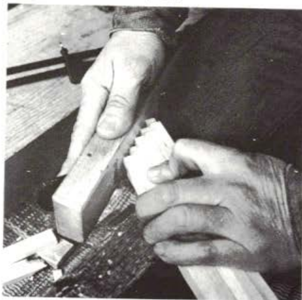
With the kumiko still clamped together, Odate makes their tenons. First he saws the shoulders, then breaks off the waste with a chisel pushed in from the end grain (top). The index finger on the bottom of the chisel acts as a stop to protect the shoulder. He cleans up the tenons by paring with the chisel across the grain (above). When all the tenons have been formed and their top and bottom corners chamfered with a few strokes of a plane, he unclamps the stack, fans out the kumiko and chamfers the other two corners (below).
