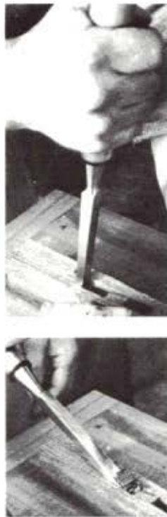
Align the chisel with the center of your body, strike it hard, and then lever out the waste.
