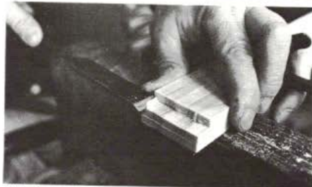
With the kumiko still clamped together, Odate makes their tenons. First he saws the shoulders, then breaks off the waste with a chisel pushed in from the end grain (top). The index finger on the bottom of the chisel acts as a stop to protect the shoulder. He cleans up the tenons by paring with the chisel across the grain (above). When all the tenons have been formed and their top and bottom corners chamfered with a few strokes of a plane, he unclamps the stack, fans out the kumiko and chamfers the other two corners (below).
