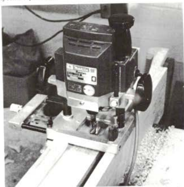
Equipped with a spiral end mill, the Makita model 3600B router is an excellent tool for mortising. But its powerful motor and square base make it also well suited for clamping upside down in the tail vise of your bench, where with the proper fence it becomes a spindle shaper.
