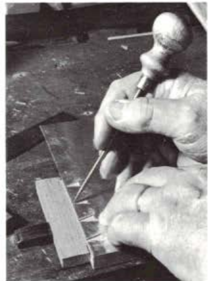
E. Marking the tail board.
