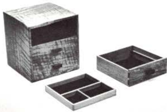
An exemplar of precise joinery, author's full-blind finger-joined music box is 4\frac{1}{2} in. on a side. Carcase is flame-figured butternut, dovetailed drawers are English beech with rosewood pulls.
