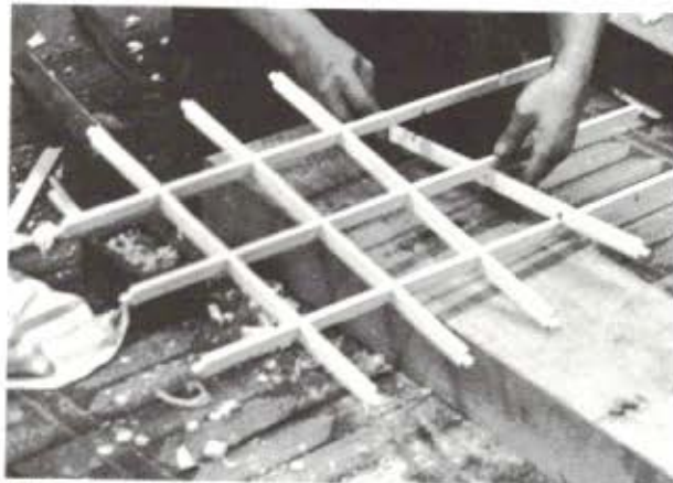
The kumiko lap joints alternate, above, and must be eased into place. Below, Odate holds a small shoji he made for demonstration during a weekend workshop.
