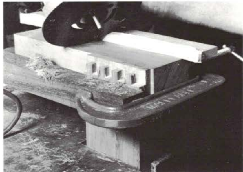
H. Routing waste for half-blind dovetails.
