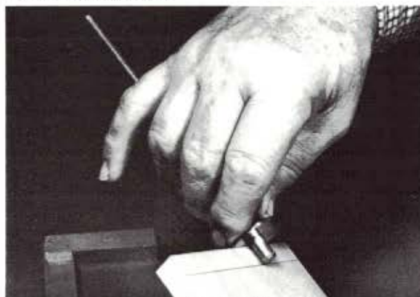
Machinist's scratch gauge marks wood and metal.
