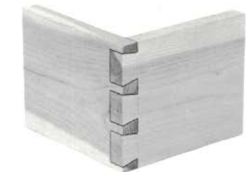
Dark veneer inlays outline the pins and tails of this decorative joint.
