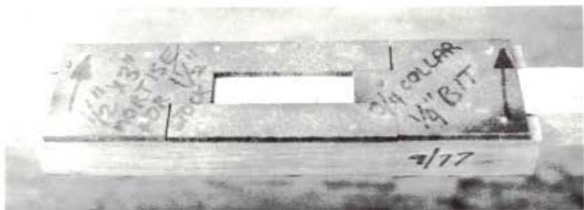
Okie's mortising jig, for use with router and guide collar, is expeditious. First lay out mortise, then clamp shoulder blocks to faces of stock, and tack hardboard template parts to blocks. Size of opening depends on offset between cutter and guide collar.
