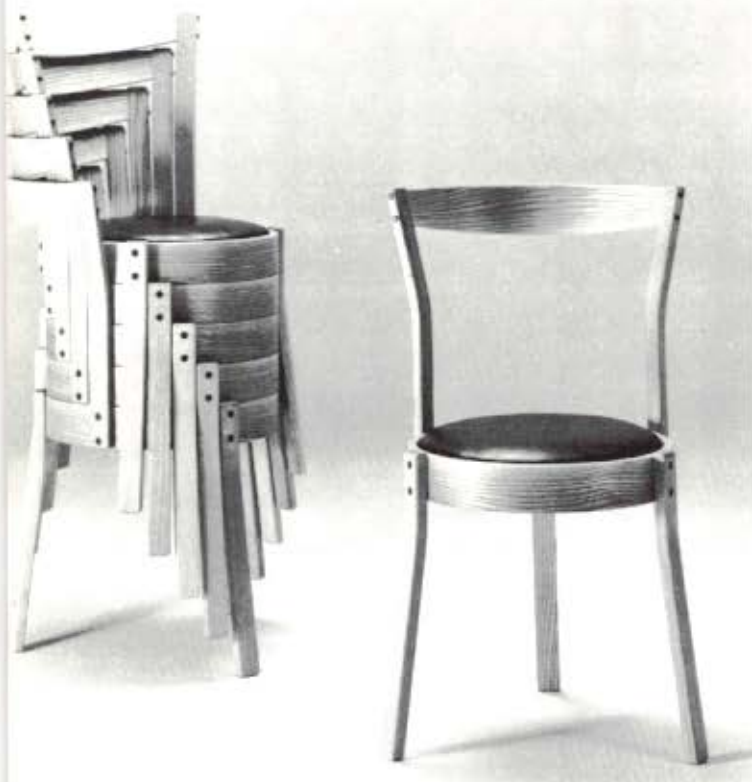
A splined key joins the ends of Erpelding's chair-seat rim at the rear leg, above. The legs are fastened to the rim with socket-head cap screws threaded into propeller nuts mounted in a reinforcing block inside the rim. The curved clamping blocks of the chair-seat rim-bending form, below, which fit inside the laminated rim when it's being glued up, are shown resting on the metal pins that align the laminates.
