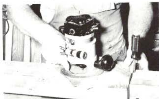
Spangler routs a slot, screwdriver indexes carriage.
