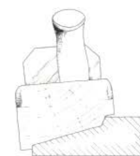
Shoulder angle is greater than 90°, thus the same plane can field panels of various thicknesses.
