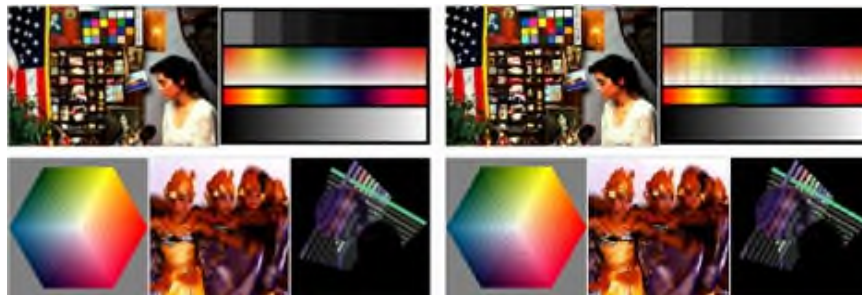
High-resolution image - Uncompressed (Left) vs. same high-resolution image - Compressed (Right). While the compressed image on the right suffers no loss in visual quality, it is represented using 6 times less data than the one on the left.
