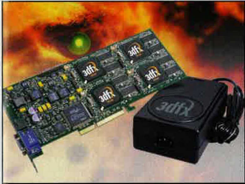
The Voodoo5 6000 draws so much current that it requires its own power adapter to assure reliable operation.
