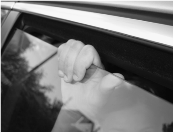
Fig. 1. A child grasps the edge of the window in the danger area between window glass and seal entry of a motor vehicle side door.
