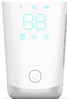
FIG. 8.1 Digital display of user interface utilizing backlit transparent housing in order to dim brightness accommodating a specific disease state in which light sensitivity is increased in patient user. Photo courtesy of HS Design.
