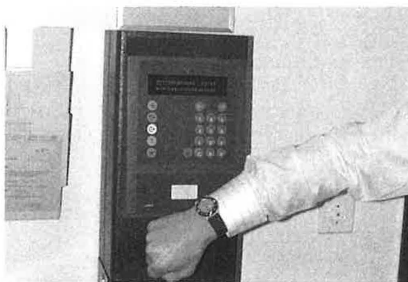
Figure 13.16 Access control and time keeping are combined in a single terminal. The watch with an integral transponder performs the function of a contactless data carrier (reproduced by permission of Legic® -Installation, Kaba Security Locking Systems AG, CH-Wetzikon)
