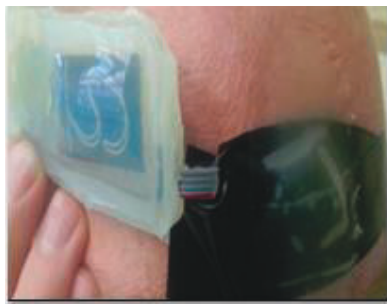
(a) Attaching the measurement unit on forehead
