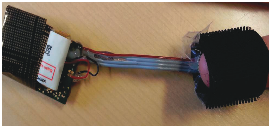
(a) Sensor attachment method for fingertip
