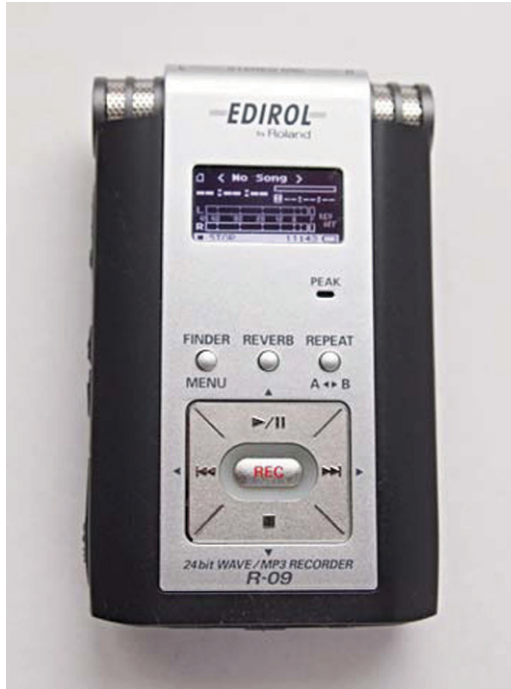
Figure 4.26 A white monochrome passive-matrix OLED display product (EDIROL R09 digital audiorecorder).
