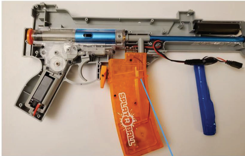
feed chamber for loading the soft-projectiles within the projectile launcher
