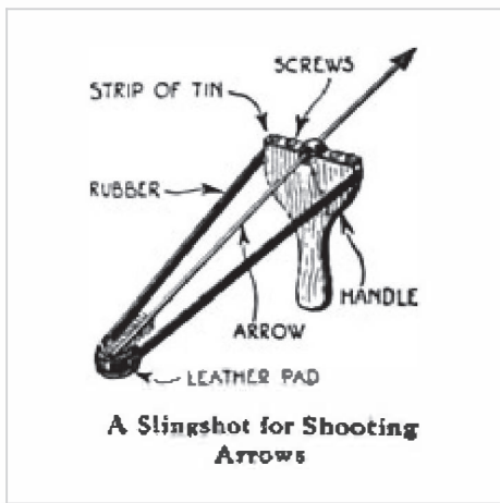
A 1922 diagram showing the construction of an arrow-firing slingshot
