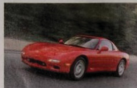
Aerodynamic car. Streamlined bodies are used for sports cars and other vehicles to reduce air drag and increase fuel efficiency. (© 1992 Dick Kelley)
