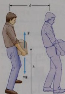
Figure 6.3 (Thinking Physics 1) A person lifts a cement block of mass m a vertical distance h and then walks horizontally a distance d .
