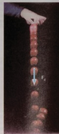
Figure 4.5 The only force acting on an object in free fall is the gravitational force, \mathbf{F}_g . The magnitude of this force is the weight of the object, mg .
