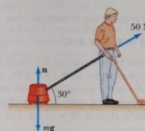
Figure 6.4 (Example 6.1) A vacuum cleaner being pulled at an angle of 30^\circ with the horizontal.
