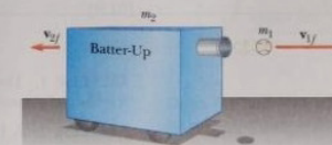
Figure 8.2 (Example 8.1) When the baseball is fired horizontally to the right, the pitching machine recoils to the left. The total momentum of the system before and after firing is zero.
