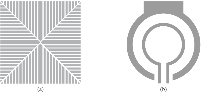
Figure 6.6 (a) A patterned shield is employed to prevent electrical fields from penetrating the substrate while preventing eddy current (closed loops) flow over a large area. (b) A co-planar ground shield improves the quality factor of the ring inductor by intercepting a fraction of the fringing fields from reaching the lossy ground.
