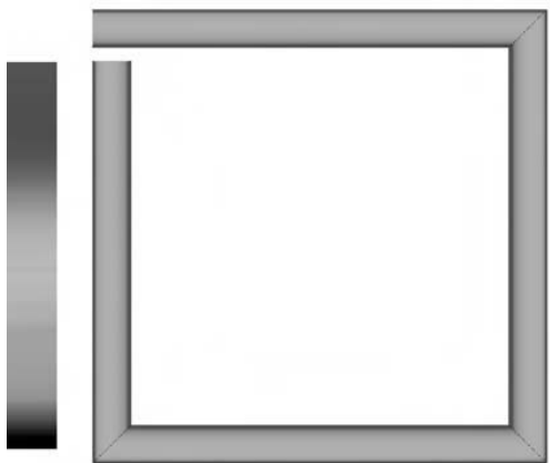
Figure 6.3 Current constriction in a square ring inductor.
