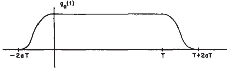
Fig. 5. Window g_a(t) multiplying all subchannel sinusoids in transmitted signal.
