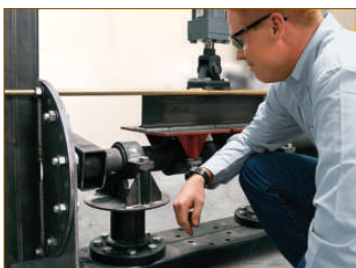
Custom-built test equipment to conduct stress tests of the bearing design
