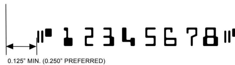
FIGURE 21 DISTANCE FROM CHECK TRAILING EDGE TO AUXILIARY ON-US FIELD NOT SUBJECT TO CUTTING AND PRINTING TOLERANCE OF PLUS OR MINUS 0.0625 INCH SEE CLAUSE 7.6.4
