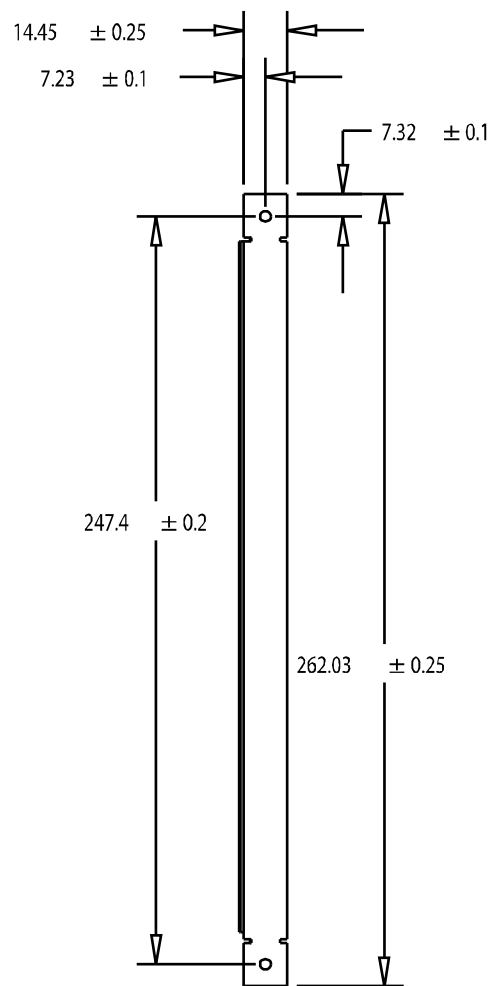
Figure 3.10-11 Unsealed Module Dimensions, Front View
