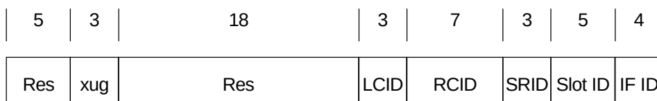
Figure 3.6-2 MAC address based on HW position
