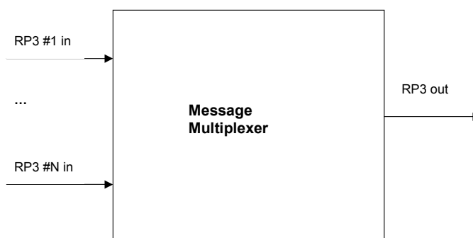
Figure 27: Illustration of message multiplexer.
