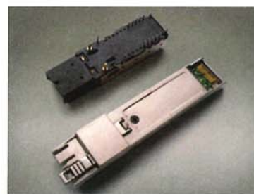
Figure 3. SFF (top) versus optical emSFP (bottom)
