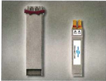
Figure 6. XFP form factor versus emSFP
