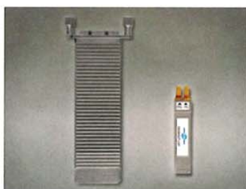
Figure 5. Xenpak versus emSFP (right)
