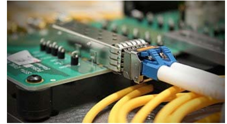
Small Form-factor Pluggable connected to a pair of fiber optic cables.
