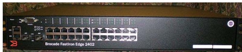
Ethernet switch with two empty SFP slots (lower left)
