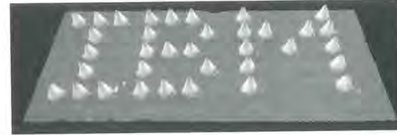
Figure 1-3 Xenon atoms individually placed on a nickel single crystal surface to spell IBM. The spacing between xenon atoms is about 1 nm. Reprinted with permission of IBM.
