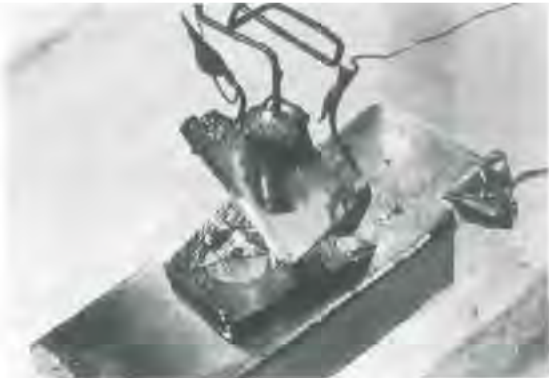
Figure 1-4 The point contact transistor invented at Bell Telephone Laboratories in 1947 by Bardeen, Brattain, and Shockley. Reprinted with permission of Lucent Technologies, Bell Labs Innovations.
