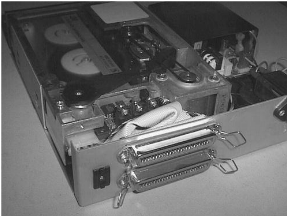
This is a typical external SCSI-1 device (a tape backup drive)
