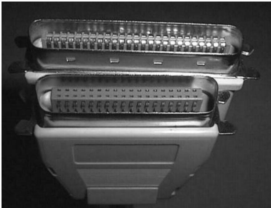
Here is a SCSI connector compared to a Centronics connector
