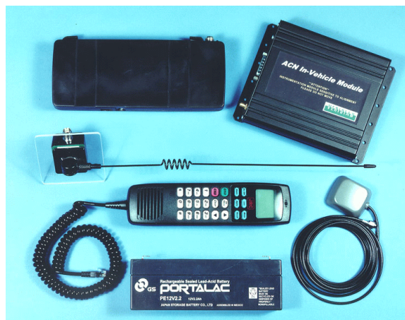
Figure 2. Veridian in-vehicle system used in the ACN FOT included a cellular phone, backup battery, cellular and GPS antennas, and an in-vehicle module with crash sensors and GPS board.
