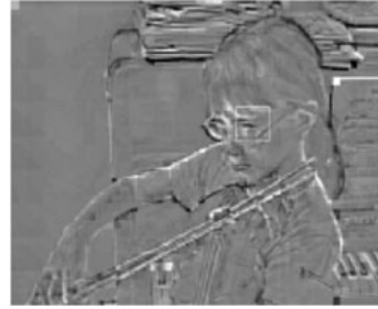
Figure 6.8 Residual after subtracting intra prediction
