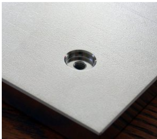
An example of a counterbore in a piece of metal
