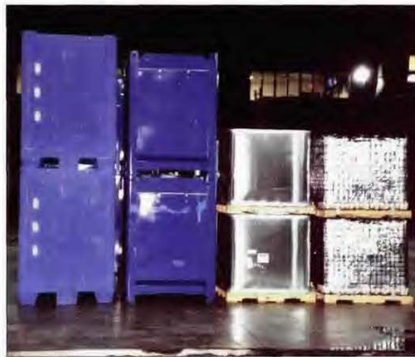
IBCs aren't easy to generalize. From left to right: two stacked sets of composite IBCs with steel outer cages, one set of stacked polyethylene IBCs with an outer layer of foam, and one set of wire-caged IBCs with a fire-resistant blanket.
