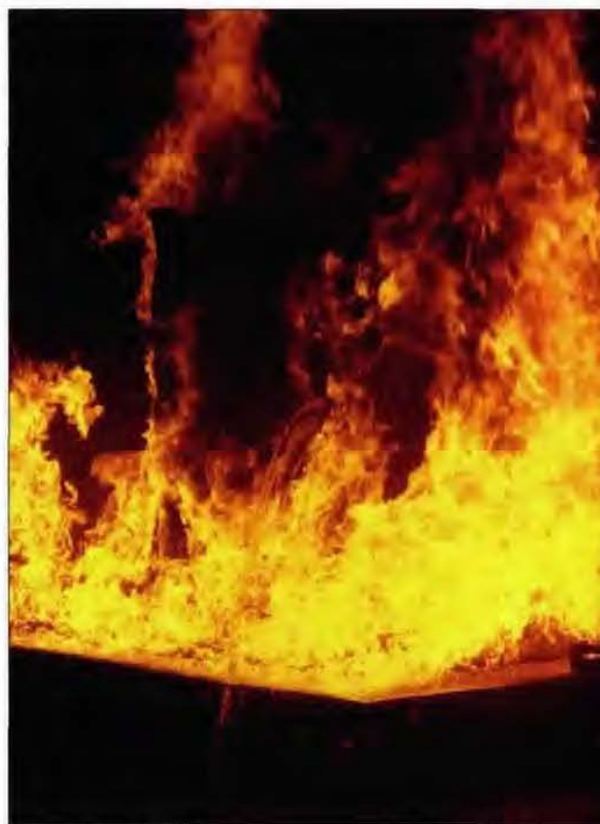
In Phase II of testing, some IBCs maintained their integrity for a full 30 minutes. Others, like this one, breached earlier.
