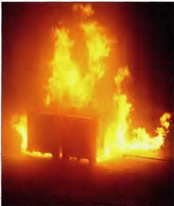
Fire tests of IBCs with sprinkler protection allowed researchers to develop design modifications to protect models like this one against leaks for 30 minutes.
