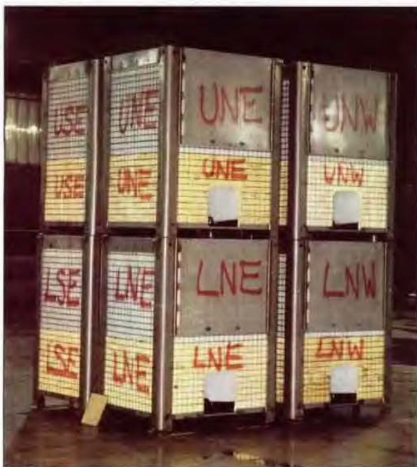
Wood sheeting was installed on the lower half of these IBCs to separate the plastic tank from the steel mesh. Fire tests showed that rotomolded units can be effectively protected by such design features that reduce full contact of the steel with the plastic.
