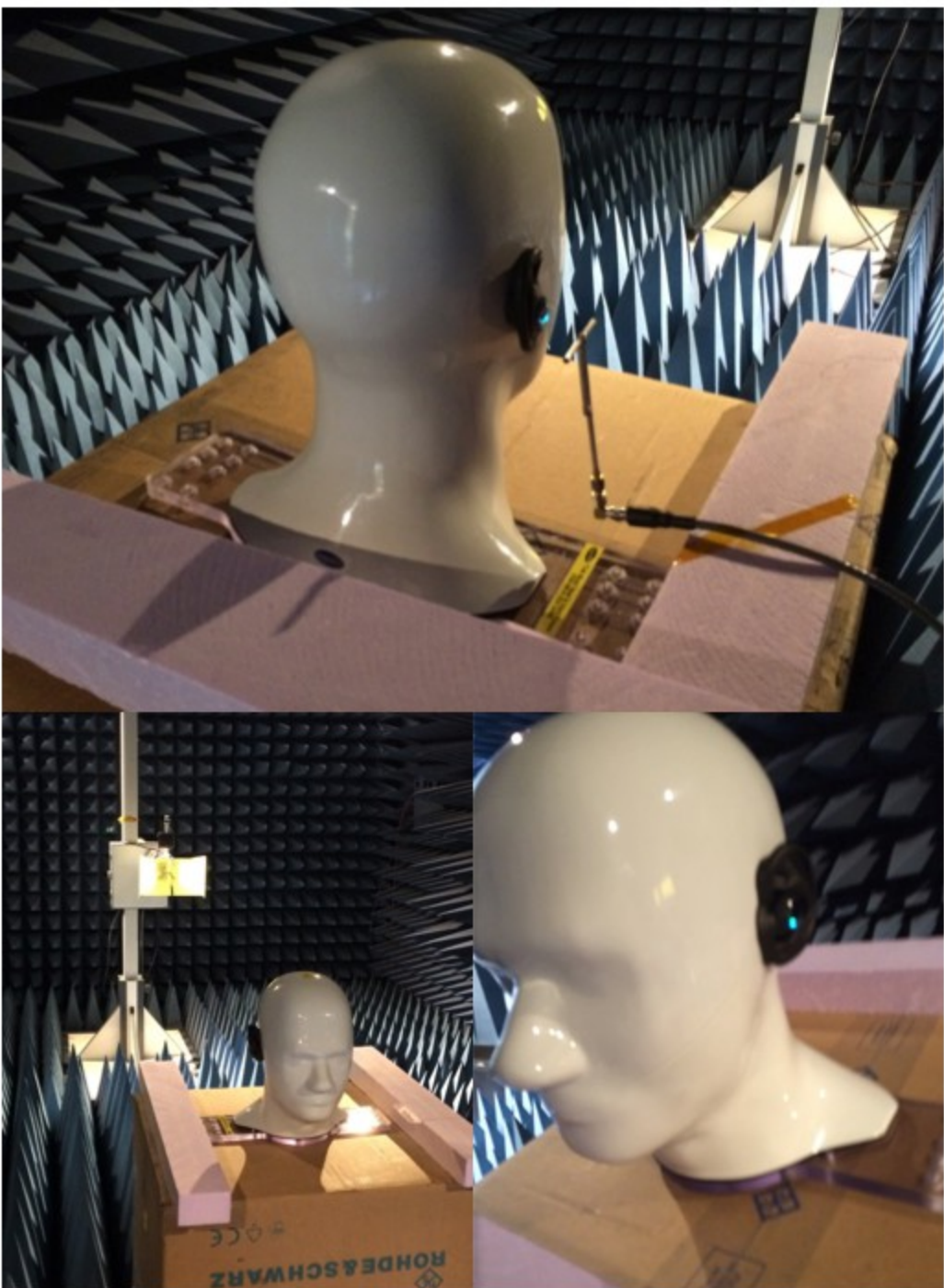
Testing wireless radio performance in anechoic chamber (reflection reduced room)
