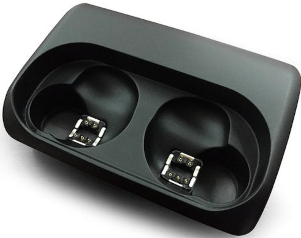
The Charging Case without the aluminium cover
