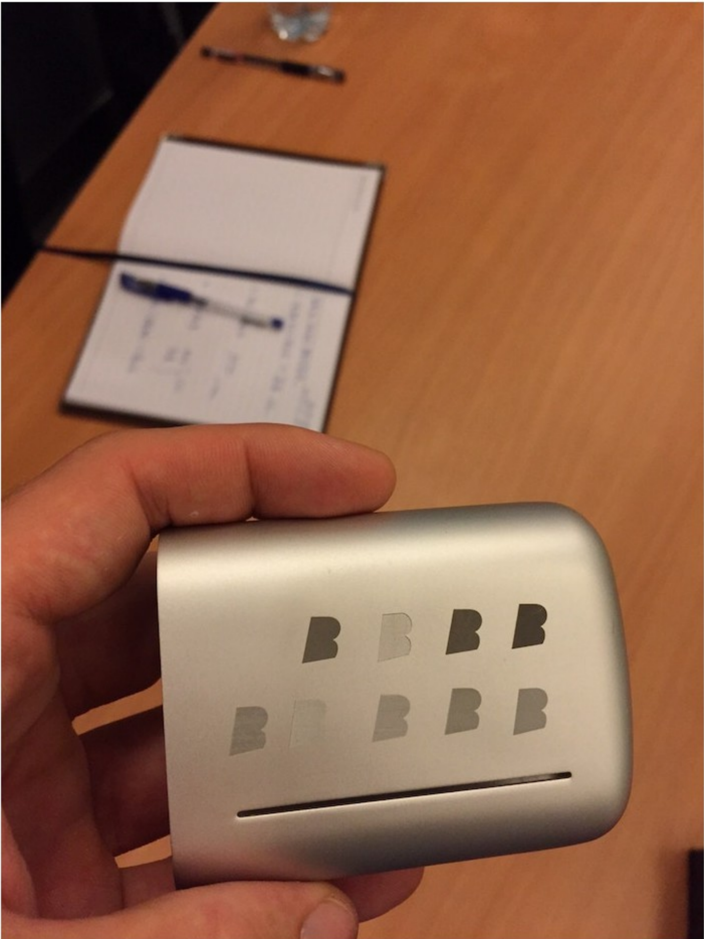
Evaluating laser engraved logo types on the aluminium case for The Case.
