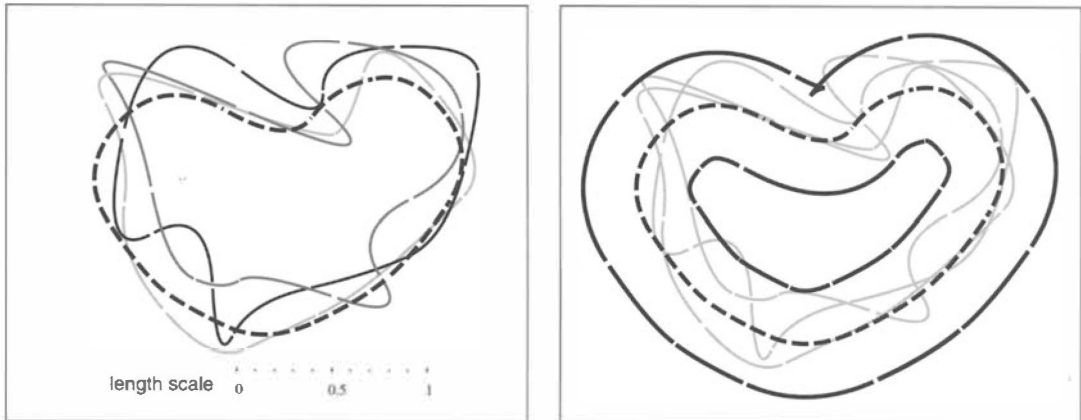
Figure 8.2: Sampling from curve families. Samples are drawn at random (left) from a uniform, isotropic, Gaussian distribution in the spline space S_Q such that \|\mathbf{r}(s) - \bar{\mathbf{r}}(s)\| has a root-mean-square value of 0.2 length units. (Mean shape \bar{\mathbf{r}} is shown dashed). Parallel curves depicting confidence intervals for normal displacement (spatially averaged), at 95% significance, contain the random curves as expected (right).
