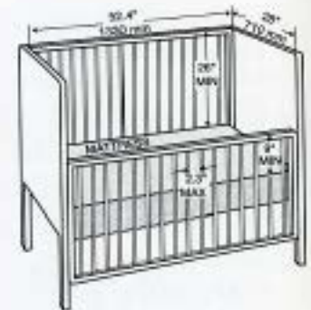
RECOMMENDED FULL-SIZE CRIB DIMENSIONS
