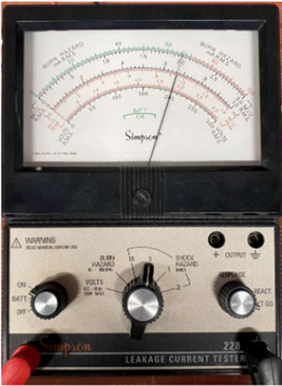
Figure 63. (Left) Relamping setup to monitor current on power loop. (Right) The Simpson 228 reads current on the power loop of the GE LED13ABT8/G4/830 LED tube lamp when the transient current is smaller than the predefined signal.
