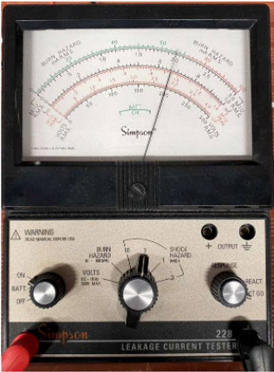
Figure 47. (Left) Relamping setup to monitor current on power loop. (Right) The Simpson 228 reads current on the power loop of the GE LED13ABT8/G4/830 LED tube lamp when the transient current is smaller than the predefined signal.
