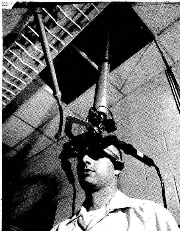
FIGURE 4—The ultrasonic head position sensor in use
