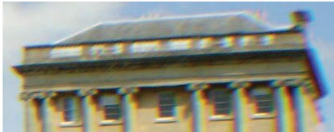
Figure 12. An example for chromatic aberration
