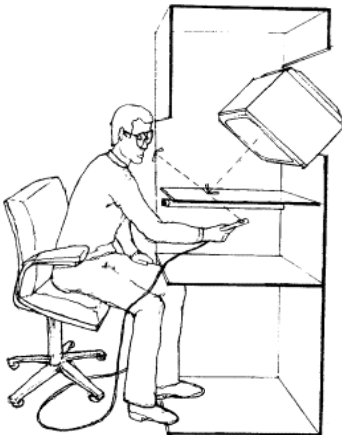
Figure 2.17: Schmandt's stereoscopic display [Schmandt, 1983] .
